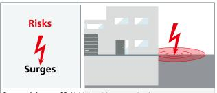
Source of damage S2: Lightning strike near a structure
